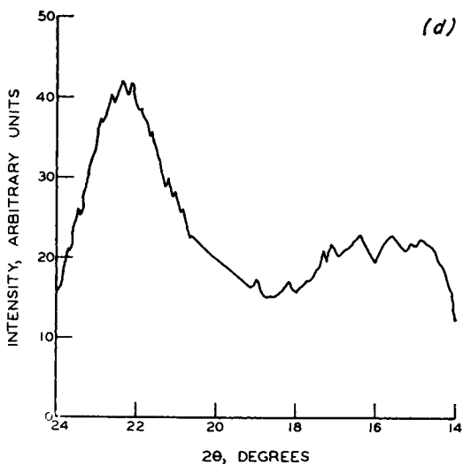
Fig. 12. X-ray diffractograms of 99.8% ethylamine treated and unbeaten cotton linters handsheets: (a) handsheet saturated with water; (b) same handsheet, partly dried; (c) same handsheet, dried more than in Fig. 12b; (d) same handsheet, completely dried.
